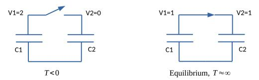
At time t = 0 the switch is closed and charge flows from C 1 to C 2 . A long time later, both capacitors reach equilibrium. They will have equal charges and voltages of 1 volt. (The total charge is the same but the capacitance has doubled, halving the voltage.)
