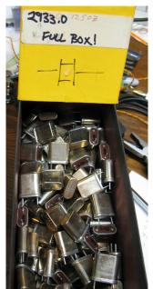
A great many of the crystals were characterized by their series and parallel resonant frequencies, series resistance and Q. Many were packaged in envelopes as matched sets for building crystal filters. Also included in the auction lot were a number of crystal oscillator circuit boards.<sup>1</sup>
