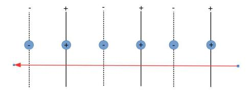
In this case we can express the signal as the vector  $\vec{Y} = [-1 +1 -1 +1 -1 +1] \cdot |y|$ . How much signal from  $\vec{Y}$  gets into  $B_0$ ? The answer is  $\vec{W_0} \cdot \vec{Y} = (-1) + 1 + (-1) + 1 + (-1) + 1 = 0$  meaning that the North pointing beam has a null at 90 degrees.
