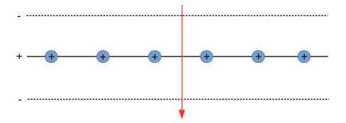
The solid line shows the crest of a southbound wave crossing all 6 elements at constant phase. The dotted lines show the troughs of the wave, which have opposite phase with respect to the crests.
