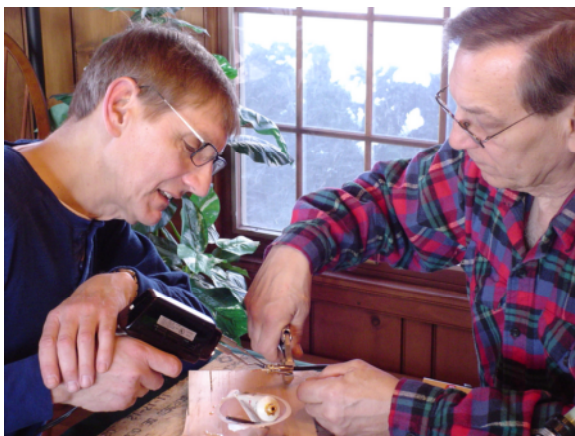
K2AL and W2IOG soldering the PL259 connector to the RG8X.
